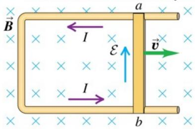
The motional emf  $\mathcal{E}$  in the moving rod creates an electric field in the stationary conductor.
