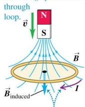
The induced magnetic field is *downward* to oppose the flux change. To produce this induced field, the induced current must be *clockwise* as seen from above the loop.
