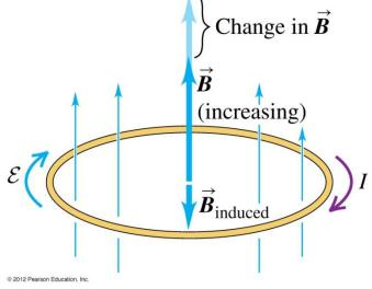
(a) Motion of magnet causes increasing downward flux through loop.
