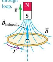
The induced magnetic field is *upward* to oppose the flux change. To produce this induced field, the induced current must be *counterclockwise* as seen from above the loop.
