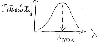
The maximum of the Intensity VS T spectrum curve is at a wavelength denoted,  $\lambda_{max}$ . The value of  $\lambda_{max}$  depends on the temperature of the Black Body:
