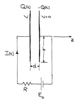
At time t = 0 a switch is thrown so that a battery, which generates emf  $\mathcal{E}_0$ , begins charging up the capacitor through a resistor. The wires that make up the charging circuit are far away from the region between the plates. The resistance R is much larger than the internal resistance of the plates, so at all times as the capacitor charges up, the charge on the plates is distributed uniformly. At time t there is a charge
