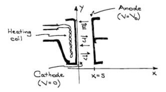
We are interested in the steady-state (time independent) "space-charge-limited" behavior of the diode. We assume that the transverse dimensions of the electrodes are much larger than s; thus we neglect edge effects and assume that all quantities depend only on the x coordinate. The boundary conditions on the potential give us
