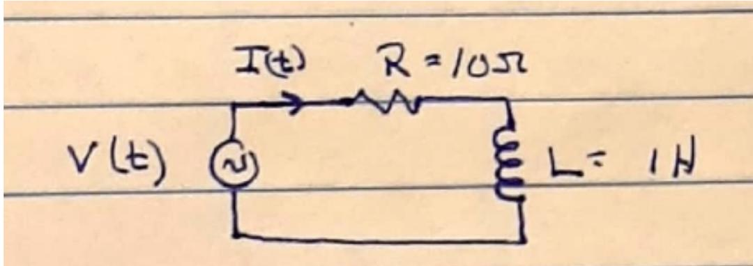
3. A sinusoidal ac voltage source  $V(t)$  oscillates with an amplitude  $\mathcal{E} = 170$  volts and a frequency  $\omega = 377$  rad/s (60 Hz). The source is connected in series in a closed loop with a  $10 \Omega$  resistor, a  $1 \text{ H}$  inductor, and a  $10 \mu\text{F}$  capacitor. The current through the capacitor is given by  $I(t) = I_0 \cos \omega t$  in steady state. Apply Kirchoff's voltage law,
