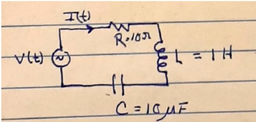
4. Carry out the calculations for problem 3 above for an arbitrary driving frequency  $\omega$ , and make a graph of the average power  $\overline{V(t)I(t)}$  delivered to the circuit versus  $\omega$ , in the range  $200$  rad/s to  $400$  rad/s. Your graph should show a peak at the resonant frequency.
