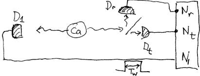
A beam splitter and a photodetector are placed equidistant from the radiating Ca source. By detecting one of these photons directly, we know that there must be exactly one photon incident
