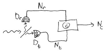
According to the classical theory, the intensity of an incident field, no matter how weak, will be equally divided at the beam splitter, and therefore, the average number of coincidence counts registered in any time window will be at least as big as the product of the number of counts registered by each detector individually,
