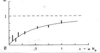
We see a violation of the semiclassical theory which requires  $\alpha \ge 1$ . The deviation from perfect anticorrelation,  $\alpha = 0$ , when the pumping rate or  $T_{window}$  is large arises become coincidence counts can arise from two photons "born" from twins at different times.
