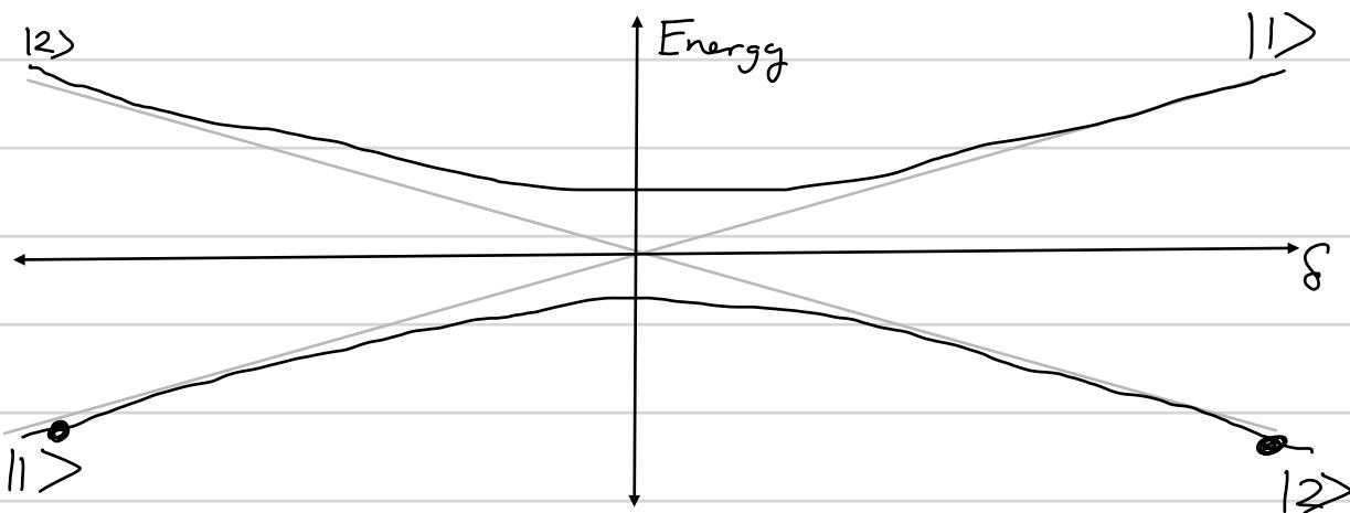
By adiabatically sweeping  $\delta$ , we transfer  $|1\rangle$  to  $|2\rangle$  in a manner that is robust to the energy difference between  $|1\rangle$  &  $|2\rangle$ . This is known as **Stimulated Raman Adiabatic Passage**, or **STIRAP**. It is effective when  $\Omega_{\text{Ran}} \gg \gamma_s$ , the scattering rate.
