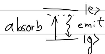
For low saturation: Photon scattering rate:  $\gamma_s = \frac{S}{2} \Gamma = \frac{I}{\hbar \omega} \sigma_{bs} = \frac{I}{\hbar \omega} \frac{\sigma_0}{1 + \frac{4\Delta^2}{\Gamma^2}}$
