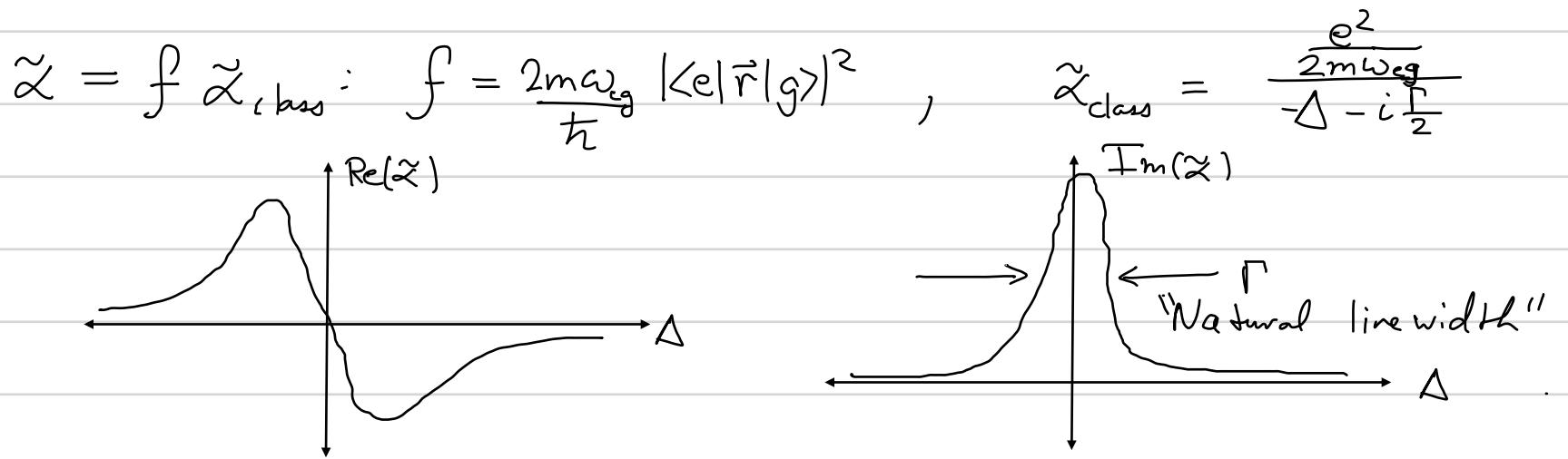
The dipole response of a two-level atom to weak driving near resonance
