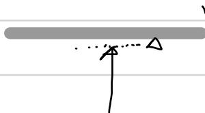
$$\begin{aligned} \mathcal{D}(E_e = E_g + \hbar\omega_L) &= \frac{\hbar\Gamma/2\pi}{(E_e - E_g - \hbar\omega_L)^2 + (\frac{\hbar\Gamma}{2})^2} \\ &= \frac{\Gamma/2\pi}{\Delta^2 + \Gamma^2/4} \quad \text{Atomic lineshape} \end{aligned}$$
