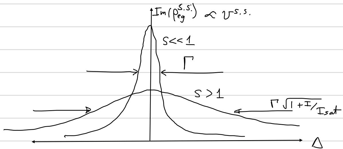
The probability of exciting the atom is "broadened" when the intensity  $I \geq I_{\text{sat}}$ . The effect is known as "power broadening."
