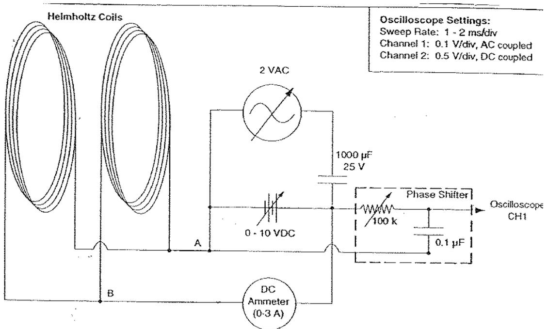
Figure 7.5: Schematic for Helmholtz coil connections
