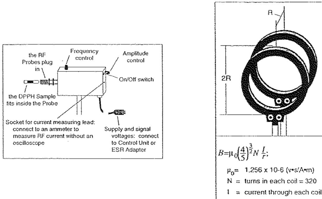
Figure 7.3: ESR probe unit (left) and Helmholtz coils (right)
