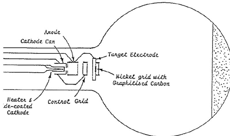
Figure 2: Schematic of the Electron Diffraction Tube
