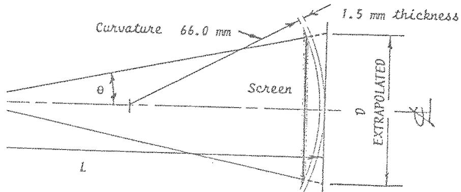
Figure 4: Curvature and glass thickness of the electron diffraction tube. The length  $L = 13.0 \pm 0.2$  cm.
