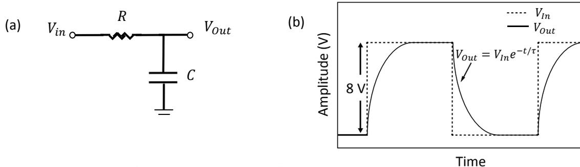
**Figure 1.** (a) RC circuit. (b) Transient response of an RC circuit.
