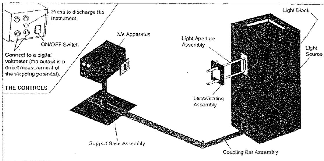
Figure 5.1: Equipment setup using a mercury vapor light source and the  $h/e$  apparatus.
