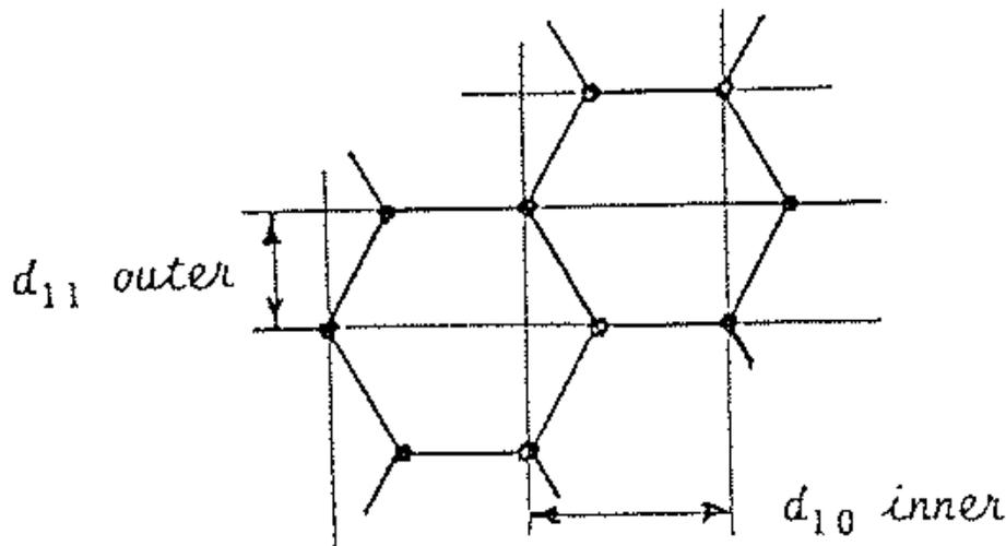
Figure 3.1: Structure of Graphite
