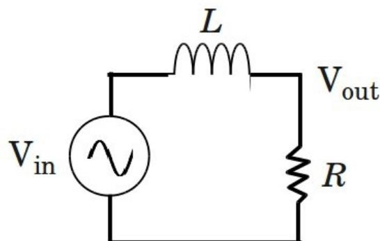
Build this circuit with the second resistor having a value of around  $1000\ \Omega$  and the inductor measured previously (in the range  $3\text{--}5\text{ mH}$ ) to produce a cutoff frequency near  $40\text{ kHz}$  (not critical) according to the formula  $f_c = \omega_c/2\pi = R/2\pi L$ . Perform the same set of measurements as with the R-C filter, but adjust your data range to account for the higher cutoff frequency. The goal is to show the frequency response rolloff with data points
