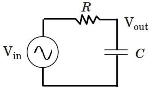
$V_{in}$  is supplied by the function generator and  $V_{out}$  is the voltage across the capacitor. Measure  $V_{in}$  on CH 1 of the scope. You can use a scope probe connected to R; clip the reference lead to ground. The less cluttered option is to use a BNC T-connector to route the function generator signal directly to the CH 1 input (i.e. scope probe not needed) and to the circuit with a BNC/EZ-hook cable. Connect a scope probe to CH 2 and clip it across C to measure  $V_{out}$ .
