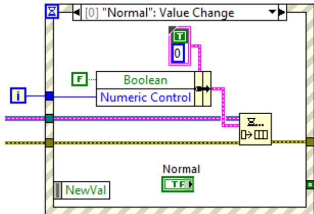
Next, build the High Priority event in the producer loop. It should be configured the same as the Normal event with the following changes: i) Boolean constant is TRUE, ii) Numeric Control is a constant  $-999$ , and iii) use instead 'Enqueue Element at Opposite End' function. The latter operation will put this event at the front of the queue, i.e. high priority events get handled before the normal events in the queue. The Stop case can remain as in the template.
