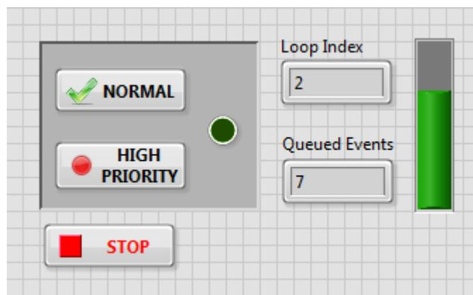
Go to the Block Diagram and edit the producer loop Event Structure. You will need three separate event cases to look for a value change when any of the three Front Panel buttons is pressed. Review LabView Assignment 3 for the procedure to configure events. Drag the Boolean icons inside their corresponding event cases.
