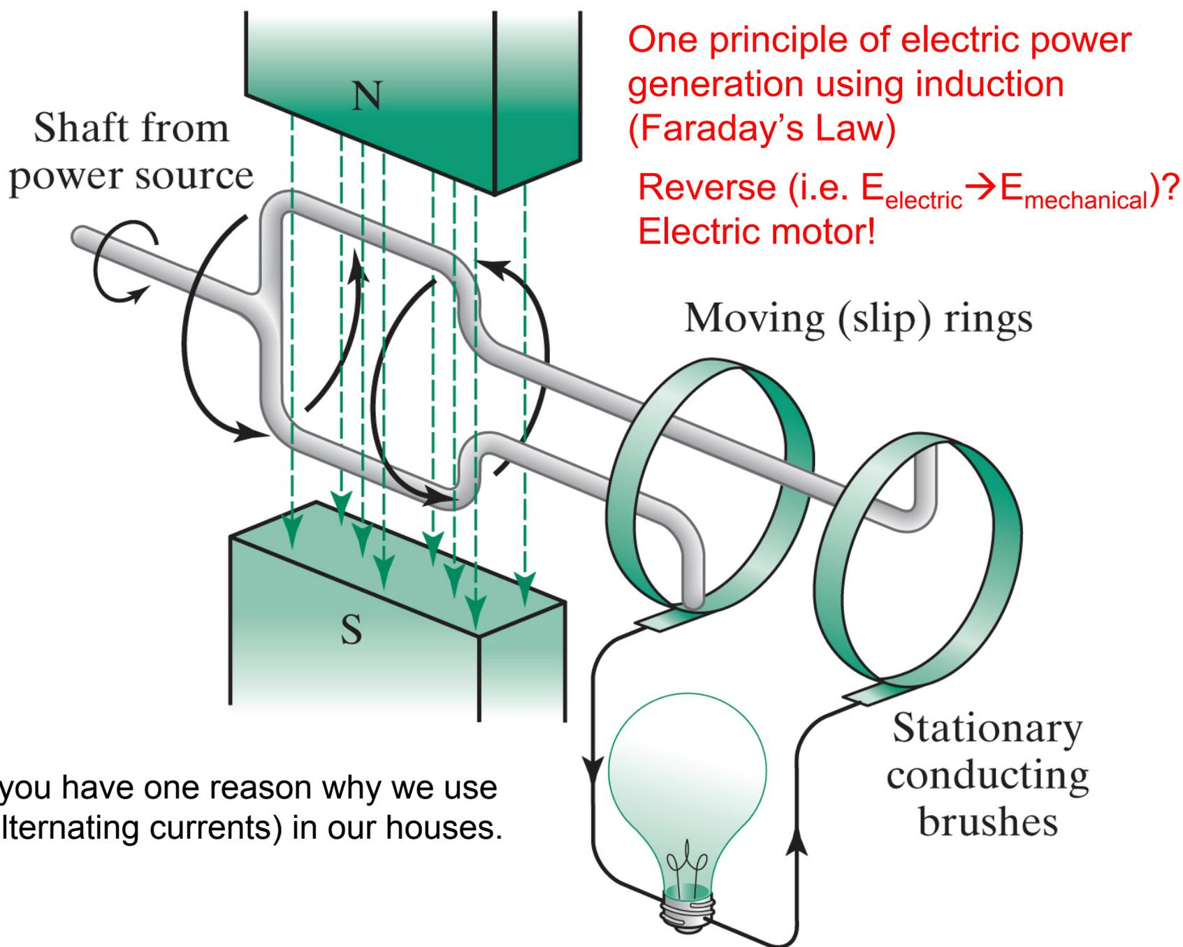
One principle of electric power generation using induction (Faraday's Law)
